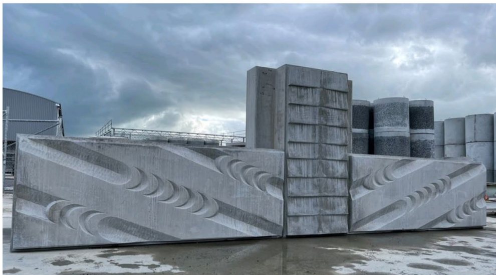
Figure 6: “Carved” concrete blocks in casting yard in Te Awamutu
