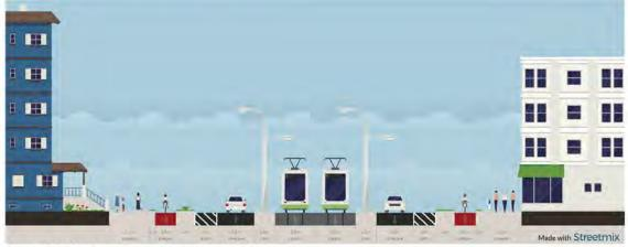
Figure 24: Northern section Option 3B - light-rail
