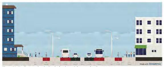
Figure 22: Northern section Option 2 - bus lanes & improved active transport
