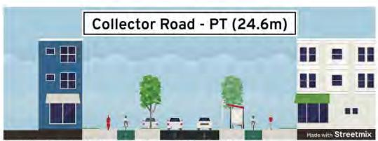
Figure 10: Proposed Collector Cross-Section for Identified PT Routes
