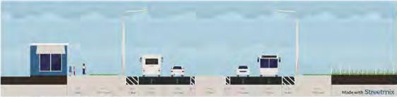
Figure 21: Northern section Option 1 - bus lane
