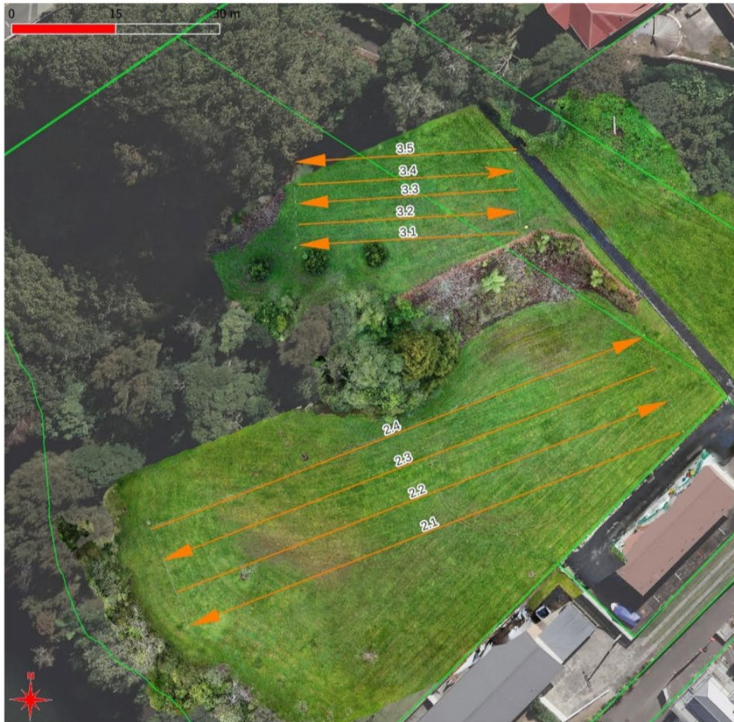
Figure 17: GPR lines on the Jesmond Park. 2024 high resolution orthophoto combined with LINZ aerial.
