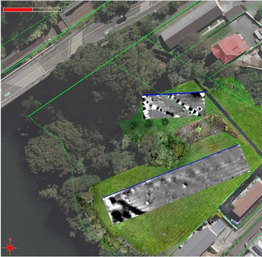
Figure 11: Geomagnetic survey grids in the park. Note the strong dark 'blobs' (anomalies) in the southwestern corner.
