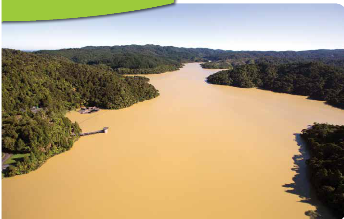
Cosseys Dam, Hūnua Ranges, was particularly hard hit during the Tasman Tempest weather event in March 2017. The sediment blocked the Ardmore water supply treatment plant for 10 days after hundreds of landslips dumped silt and sediment into the Hūnua reservoirs. The worst-affected dams were those that had recent commercial forestry activity. Photo: Watercare
