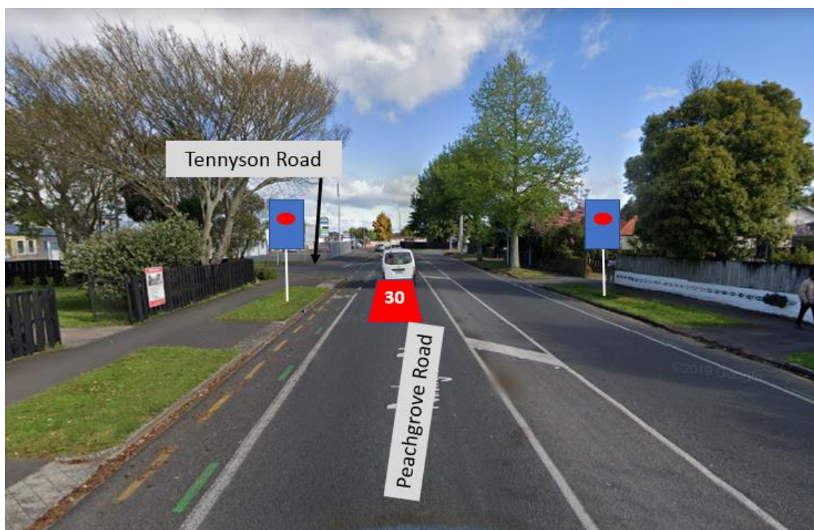
Figure 6: Illustration of new location of signage and roadmarking on Peachgrove Road
