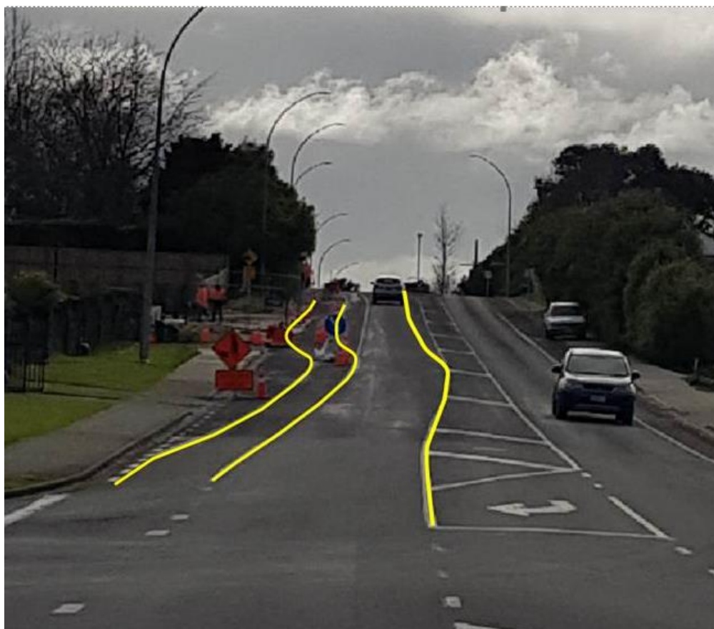
Figure 3: Illustration of cycle lane markings looking north up Horsham Downs Road from Moonlight Drive if on-street parking were retained.
