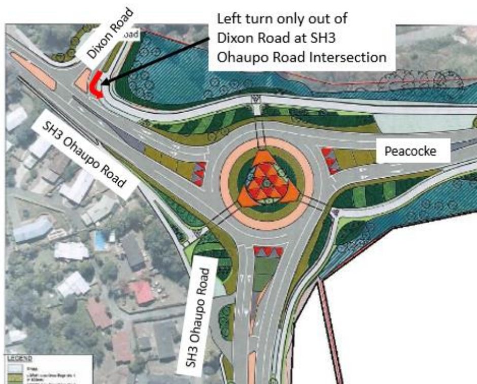
Figure 4: New Roundabout on Ohaupo Road and proposed right turn ban out of Dixon Road
