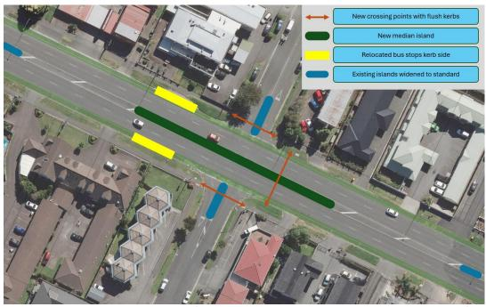
This option partially mitigates the risk for pedestrians and crossing the road to access Abbotsford Street and the local bus stops. The crossing includes a widened median island to provide safer and more comfortable place for pedestrians to wait while crossing. The crossing is closer to the desire line for pedestrians which will encourage pedestrians to use the facility rather than crossing informally.
