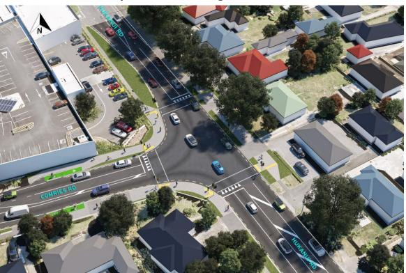
Signalised intersection would allow both active mode users time to cross the intersection and reduce delay for buses.
