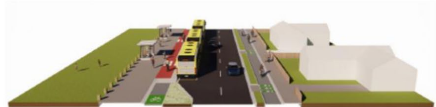
Figure 4-3: Oblique Perspective Showing Typical Section of the Preferred Option on Peachgrove (20m) Outside a School
