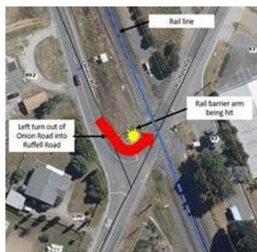
Fig. Two: Truck turning movement out of Onion Rd
