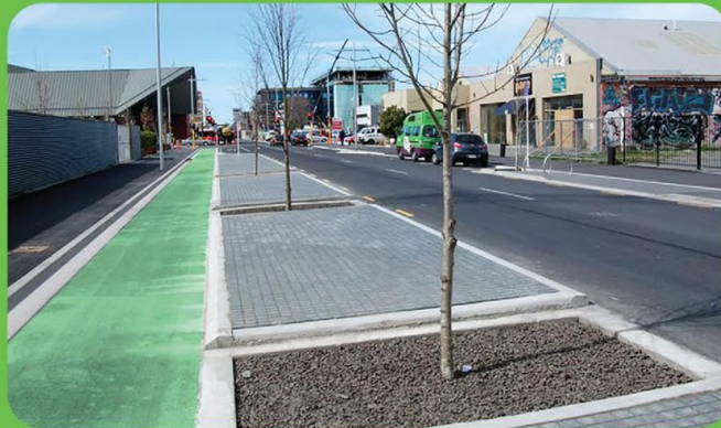
Separated bikeway with physical barrier
