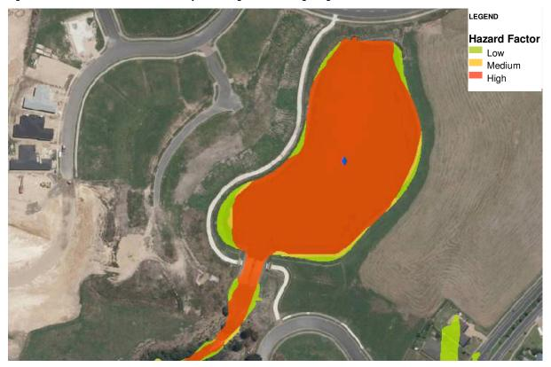
While flow rates through the lake are expected to double for the future scenario, the lake level is expected to increase by only about 300 mm. The additional flow volume is likely to be managed effectively through the lake due to the lake volume and the effect of the outlet control structure.
