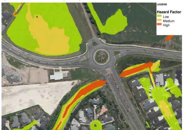
While the flows increase significantly for the future scenario, flows are predicted to be contained within the floodway extents. Future development in the upper catchment is expected to result in flows being re-directed along roadways. Some surface ponding is still predicted to occur in the upper catchment; however this is reduced compared to the existing scenario.
