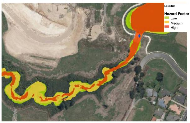
Flows across the outlet weir of Magellan Lake are expected rise about 700mm between the existing and future scenarios. Flood water is expected to be contained within the structure, however the flow velocities are likely to increase by about 20% as the discharge increases for larger storm events and development scenarios with more runoff.
