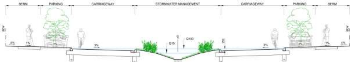
Figure 3.6A-5 INDICATIVE COLLECTOR ROAD CROSS SECTION WITH CENTRAL SWALE
