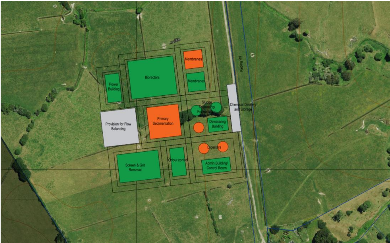
Figure 10: Early concept layout for Site 1 showing key process units for a 200,000PE plant. Processes colours orange not required until post-Stage 3.
