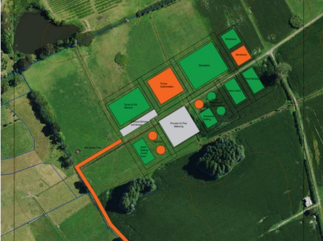
Figure 25: Early concept layout for Site 2 showing key process units. Processes colours orange not required until post-Stage 3.
