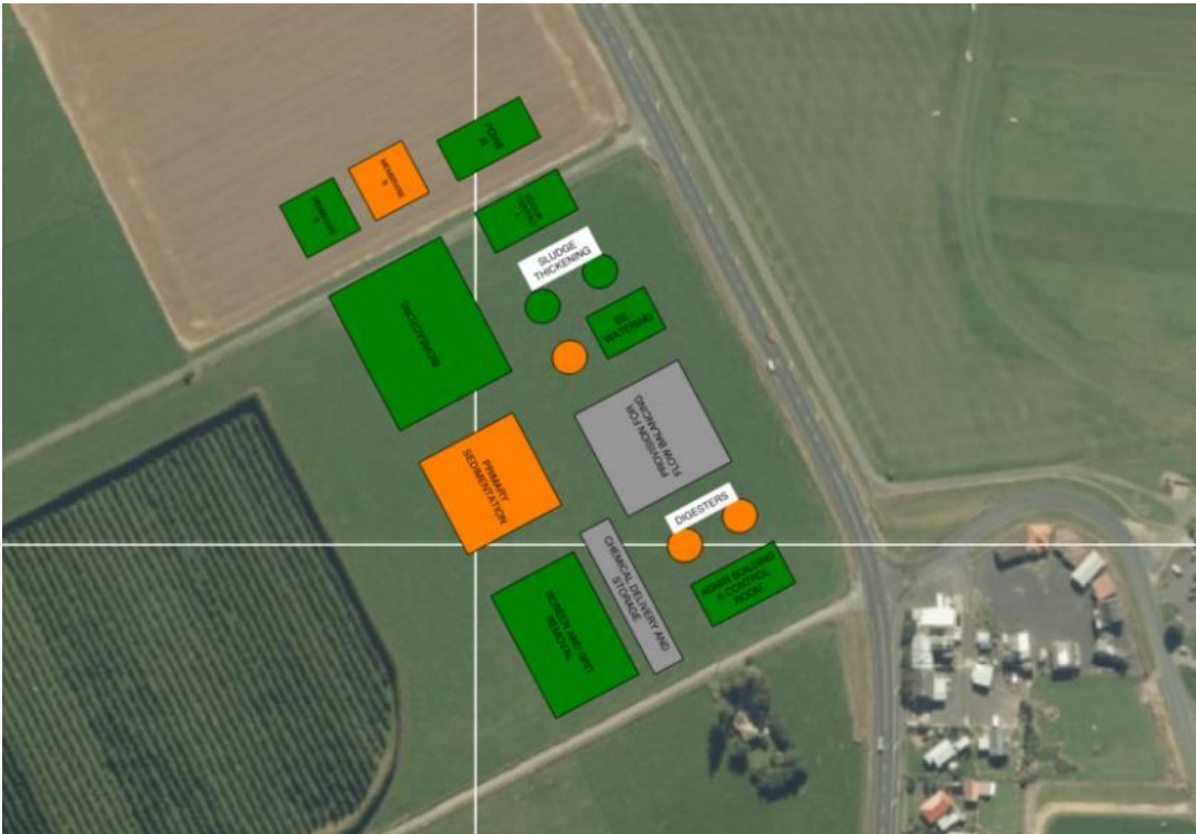
Figure 37: Early concept layout for Site 3 showing key process units. Processes colours orange not required until post-Stage 3.
