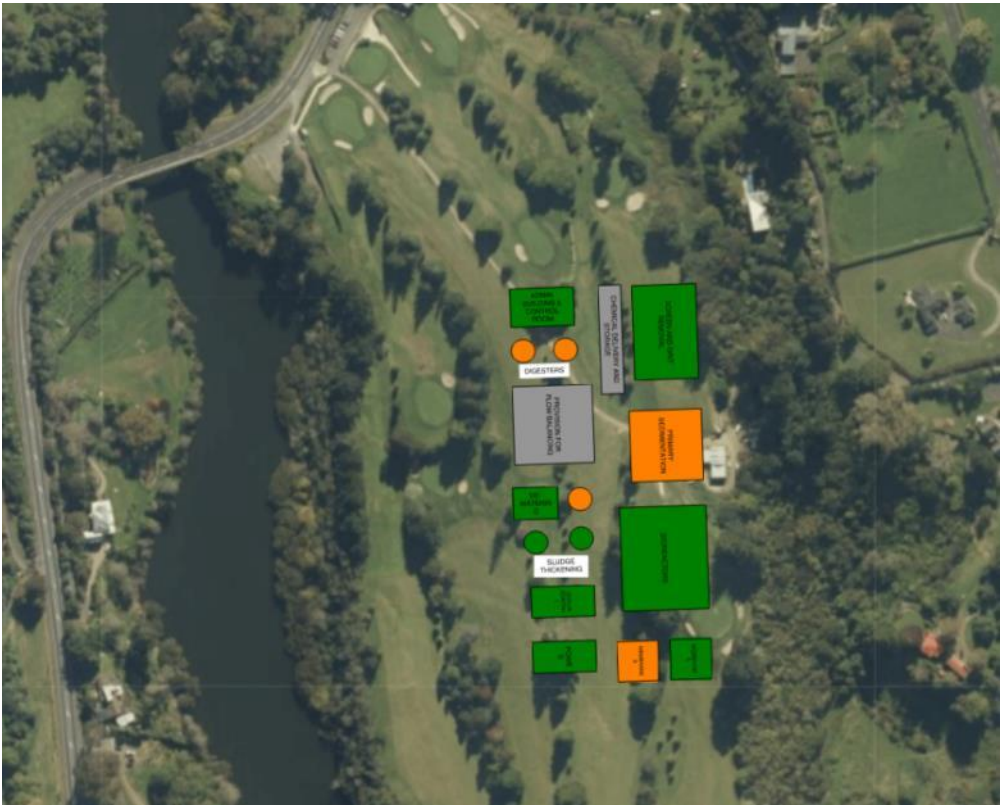
Figure 48: Early concept layout for Site 4 showing key process units. Processes colours orange not required until post-Stage 3.
