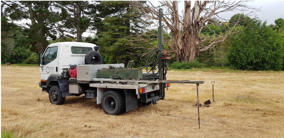
Figure 1. A light coring rig was used to obtain an undisturbed soil core for description where crop damage was not of concern.
