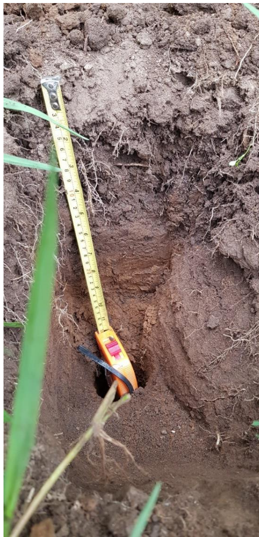
Figure 13. On elevated rolling land at the Narrows Road site, soils are developed in clayey Hamilton Ash which is very firm.
